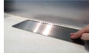
The power point S-Box presents three standard sockets at the touch of a finger from their 'secret' position in the work surface. Ideal for open-plan kitchens or island features, or simply where good design is important. A separate switch activates or isolates all 3 sockets. The cable tail provided (emanating from the housing below) should be connected to a surge-protected junction box by a qualified electrician.
